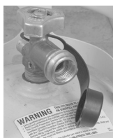
(B) Nipple has to be centered into the LP tank valve
