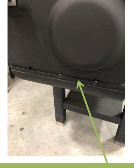
Please note that when installing the bottom panel back into place, you will want to make sure this lip is tucked inside the panel before tightening your screws on the bottom.
