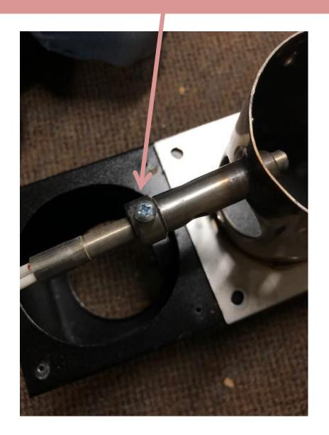
To install the new hot rod, you will need to remove the blower fan and then feed it through the auger shaft. To do this, there are just 4 more screws to remove. Once you feed the hot rod down the shaft, place the clasp through the hole, you pushed the old one through on the side of were the fan mounts.
