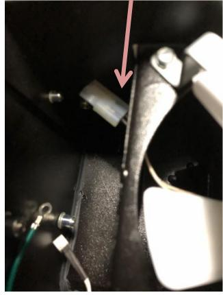
Now move back to the burn cup. Please note, where you have the clasp pushed through the hole, you will have less room to work with. Do not pull to hard on the hot rod, or you will pull the clasp off. Bring the burn cup to the opening and install the hot rod so it is out about a half an inch to a quarter of an inch. Tighten the set screw and then angle the burn cup back in. Once the burn cup is in place, you can tighten the screws.
