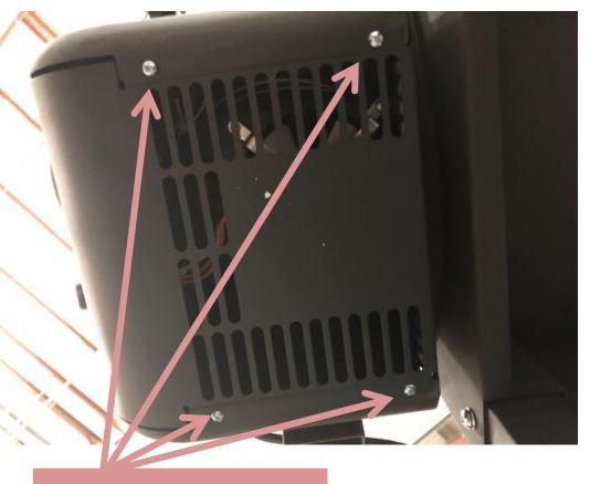
To take the bottom panel off the hopper, unscrew the 4 screws on the bottom of the hopper.
