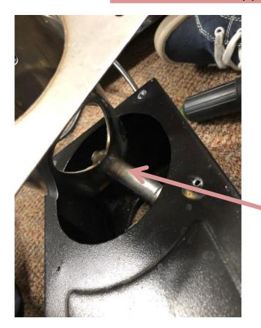
When the 4 screws are removed, angle the cup out, to get to the hot rod.
