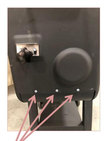
Then take out the 3 screws on the left side of the hopper. At the bottom of the side panel.
