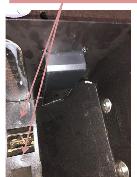
Next there is 2 screws on the front of the hopper on the right side, and 2 screws on the back of the hopper on the left side we will take off.
