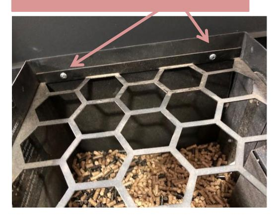
Once the screws are moved, you will pull up on the guard up and then it will lift off of this ledge.
