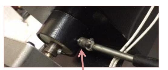
If you are changing out the bushing, you will need to remove the self tapping screw from the auger bushing. Once you remove the screw, the auger and bushing will slide out.
