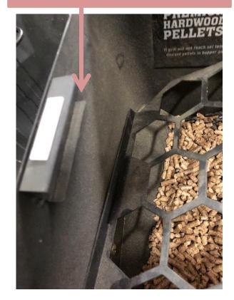
Once the guard is off and the pellets are emptied out, there is two screws at the bottom. Remove these 2 screws.
