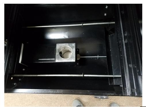
Once you pull the heat deflector off the rod, you can clean out the bottom of the pellet grill and\or change out the part.
