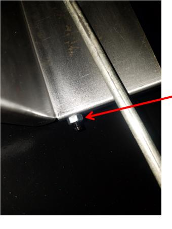
Once you get that first nut off, you can pull the heat deflector forward to get to the other nut. Once you get the second nut off, you can pull the heat deflector off of the rod.
