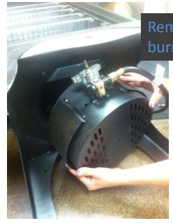
Remove the burner Drum
