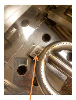
It is connected by this 1 screw. Once you take out the screw, the burner will pull out from the valve.
