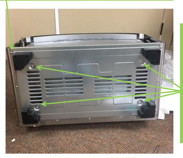
There are 4 screws in the middle that you will need to remove as well. Again, these screws are different than the ones around the out side piece of the bottom. (The feet do not need to come off)
