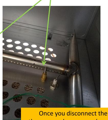
thermocouple you can place the new one in and re assemble. You can do this by following the directions in reverse.
