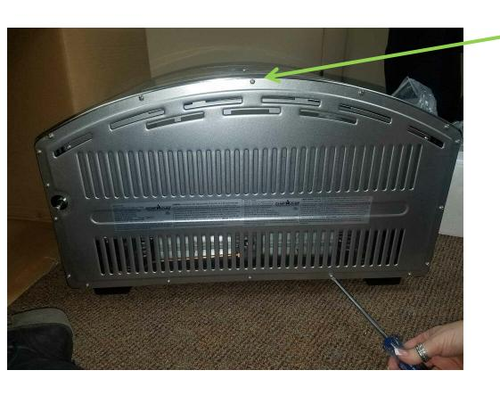
The first thing is to take all the screws out of the back. They will be all around the back side. There is 17 total. Please note that there are a couple different type of screws and you may need to make piles that are labeled.
