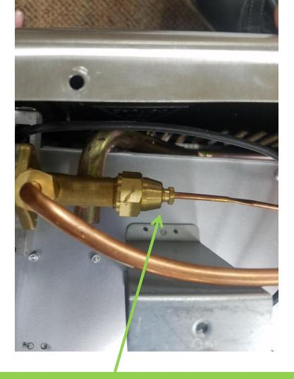
You will then want to disconnect the thermocouple from the valve.
