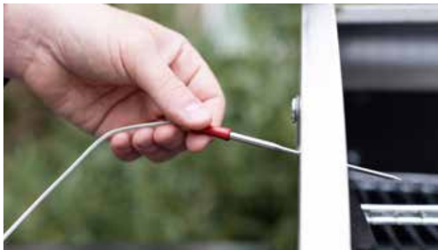
12. Insert the probe and wire through the stainless flap on the side of the chamber.
