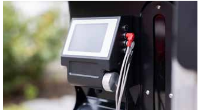
11. Plug the probe into one of the four available ports on the controller.
